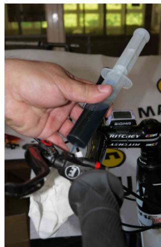
In the last step pull the piston above the hole at “30” on the scale. With this the system will be pressureless, Press your finger on the hole in the syringe and remove the syringe.
