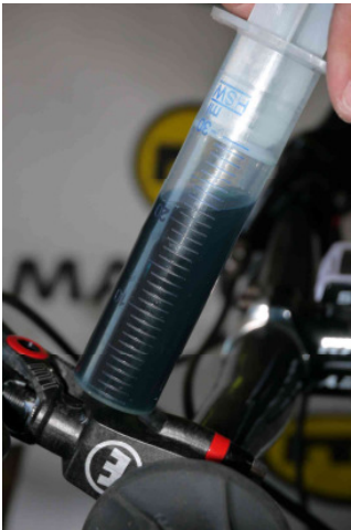
Pull the piston up to “30” on the scale, just below the hole, press in the oil again in the master Repeat this about 3 - 4 times.
