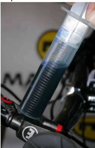
In the last step pull the piston above the hole at “30” on the scale. With this the system will be pressureless, Press your finger on the hole in the syringe and remove the syringe.
