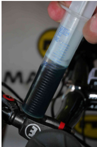
Pull the piston up to “30” on the scale, just below the hole, press in the oil again in the master Repeat this about 3 - 4 times.
