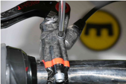
Remove the EBT screw with a Torx T25
