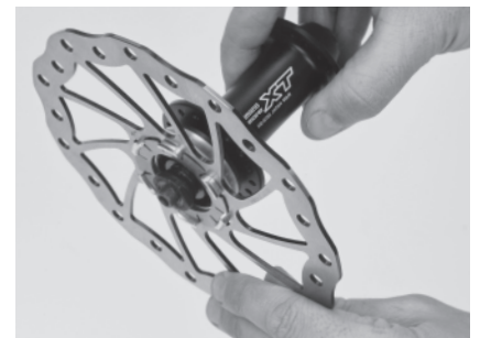
3. The prepared SL-rotor is mounted onto the hub and secured with the lock ring.
