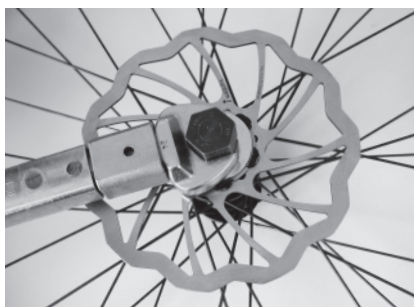
4. Tighten the lock ring with an appropriate tool (e.g. Shimano TL-LR 15). Tightening torque: 40Nm/340 in.lbs.
